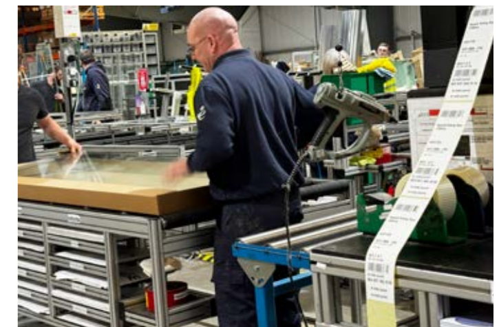
PRODUCT TRACEABILITY Roman take digital photographs of each product in production and each box has a unique code for 10 years.
