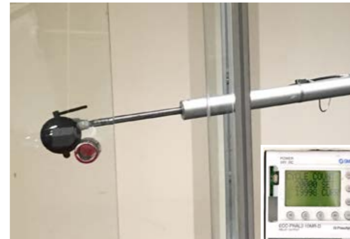
ENDURANCE TEST The shower door is open and closed on a 20,000 cycle to ensure endurance.
